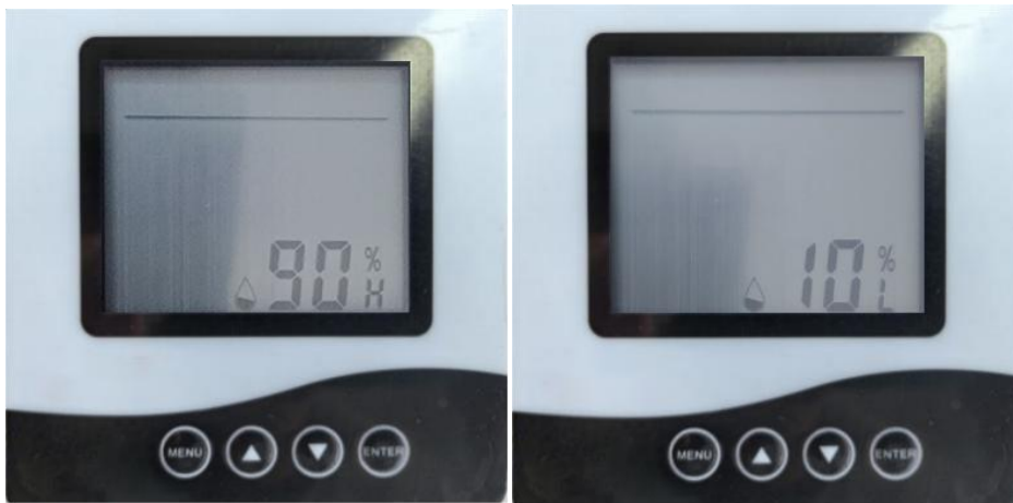
Figure 5: Setting Humidity Upper and Lower Limits on the Sensor (The setting on the left marked with 'H' is for the upper humidity limit, and the one on the right marked with 'L' is for the lower humidity limit.)
